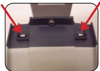
Make sure the contact points of the control box and the battery are not damaged or corroded. If there is corrosion clean with Scotch-Brite™ pad. Put some dielectric grease on the contact points before reattaching the battery.
